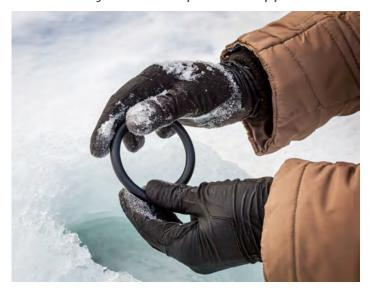
Freezing conditions can be harsh on elastomeric seals. As temperatures drop below the material's capabilities, elastomers can become more plastic-like. This change leads to reduced flexibility, increased brittleness, less rebound, and a diminished ability to maintain a proper seal.
